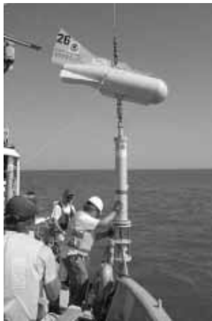
Information from a wide variety of data-gathering techniques, such as this Vector Averaging Current Meter being deployed in Lake Michigan by NOAA personnel from the R/V Shenehon, will be tied together and made more accessible through GLOS. Photo: NOAA Great Lakes Environmental Research Laboratory.
