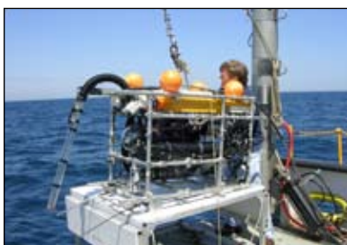
Preparing a Remotely Operated Vehicle to study lake trout reproduction on deep reefs. Photo: Bill Horns, Wisconsin Dept. of Natural Resources.
