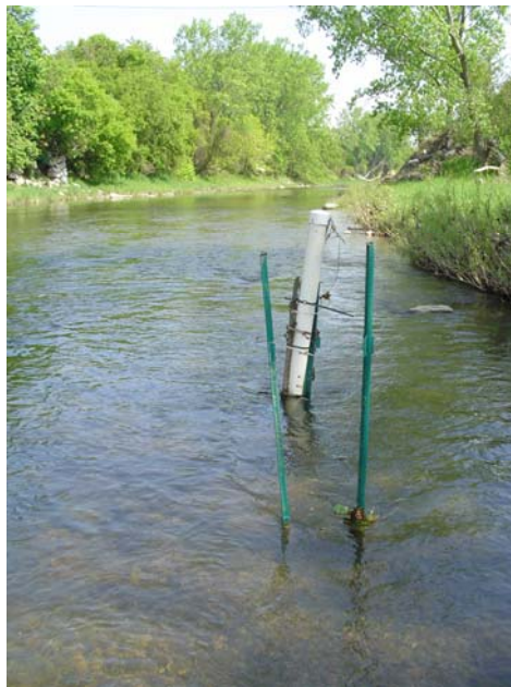
Figure 2.2: Photo showing the positioning of the YSI sonde at the watershed outlet of Cazenovia Creek (location 1A). The YSI sonde is encased within the white PVC pipe.
