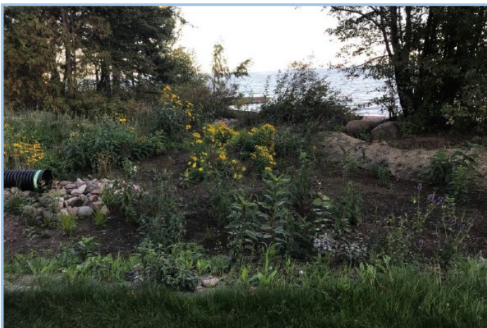
Cook County SWCD installed rain garden and bioswale projects which improve local stormwater management and capture sediment.
